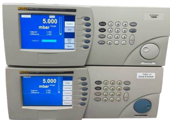
Low pressure controller, Range -75 to +75 mbar, having an uncertainty \pm 0.01\% rdg
